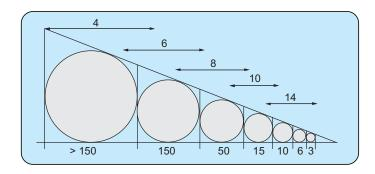
14 teeth/25 mm - cutting of thin materials of all types as tubes, pipes, profiles etc.
